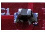
4. Repeat the process for the surface mount capacitor C1. Tin the pad, place the cap, hold it down while you touch the joint with your iron, then solder the other end.
