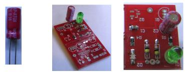
9. Next step is to install the through-hole capacitor (C2). Be careful with the orientation of this one too; the stripe on the can indicates the negative terminal, and it should be positioned in the orientation shown in the left hand photo (i.e. stripe facing "inwards"). Push it all the way down, flip the board over and solder both leads. Trim close to the board.
