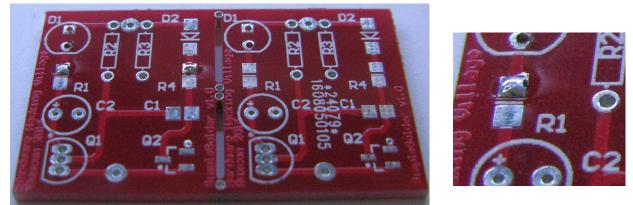
2.First we're going to solder the two surface mount resistors R1 and R4. The easiest way to do this manually is to "tin" one of the pads which basically entails applying a small amount of solder to the pad. (It's easiest to use fine solder for surface mount and thicker solder for through-hole parts) In the above image the topmost pads of R1 and R4 have been "tinned".
