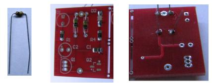
7. Grab two of your resistors and bend the leads at 90 degrees a few millimeters away from the body (left hand photo above), then insert them into the footprints on the board (R2 and R3). Once again, notice that they are installed such that they read (black brown yellow gold 100k 5%) the same way as the other components in this orientation on the board. Then flip the board over and solder the connections. Finally trim the leads off close to the board. Put one of your "pigtails" aside.
