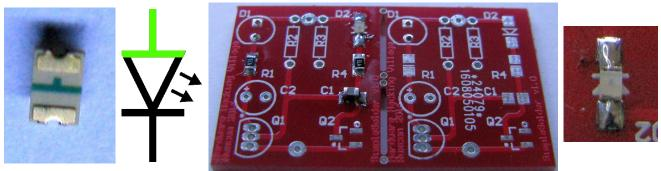
6. Make sure you orient the LED the right way around. If you look at the BACK of the LED you'll see a "T" shaped marking. That "T" shape corresponds to the highlighted "T" shape on the LED symbol next to it, which in turn corresponds with the marking on the PCB (this is the reverse of what it should be, it seems that Osram screwed up the markings on this batch of LEDs).
