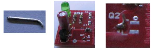
11. Now we get back to Q2. Take one of the "pigtails" you cut off earlier and put a bit of a bend in the end. Now, solder it down to the lefthand pad of Q2 (easiest to tin the pad, tin the wire, bring them together and then just a touch with the soldering iron) so that it's pointing straight up. Don't bend it around too much or you'll lift the pad off the board.
