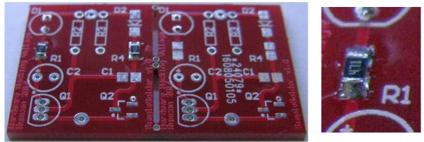
3. Next, place the resistors, positioning them so that one end is sitting on the tinned pad. Hold them in place with tweezers, then touch your soldering iron to the pad and the end of the resistor. The solder should flow onto the end of the resistor. Hold it in place for a moment while the solder freezes. After you've soldered the "tinned" end, apply solder to the other end of the resistor. Just a little dab will be enough; the end result should look similar to the above image.
