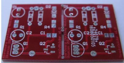
1. Each board is actually two boards. This guide only goes through populating the left hand board; the intention being that you can go and populate the right hand board yourself later (the boards can be snapped down the middle).
