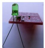
8. Next we're going to mount the through-hole LED. The holes in the design were too small for the leads of the LED so they had to be drilled out. This means that you will need to solder the LED on the TOP side of the board.
