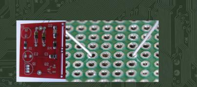
Insert your part through the appropriate holes in the PCB
