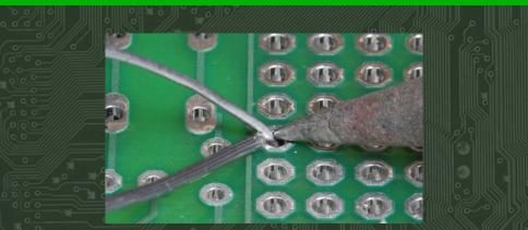
Feed in enough solder to make the joint
