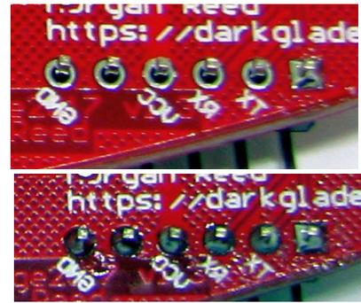
9. Next, the 6-way UART header. The “short” part of the pins passes through from the top of the board, solder one of the pins, then adjust the alignment if necessary and solder the rest of them.
