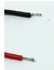
12. Last part now, the battery holder (I'd have preferred to use a PCB mount battery holder here but nobody on eBay seems to sell them in PCB mount). The leads on the battery holder are WAY longer than they need to be, trim them to about 5cm (You can get away with shorter but it makes it fiddlier), strip the ends and “tin” the wires (Apply a small amount of solder to them to make them “solid”).
