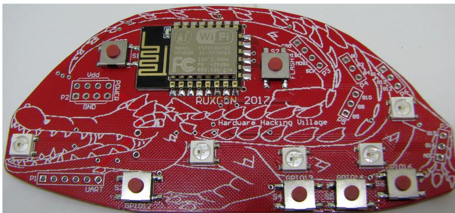
8. Next we fit the other four buttons. Repeat as for step 6 above. You'll need to take a bit of extra care with the top left pad of S6, as it's very close to LED4. If you touch the LED's body with the soldering iron, it will melt a bit. Most likely it will still work but melted components are ugly so take care ;)
