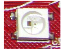
7. Now for the LEDs, notice that one corner of the LEDs have a “chamfer”, this chamfer lines up with the angled line on the PCB footprint. Same story as elsewhere here, tin one pad, tack part in place, tweak as needed, solder other three connections.
