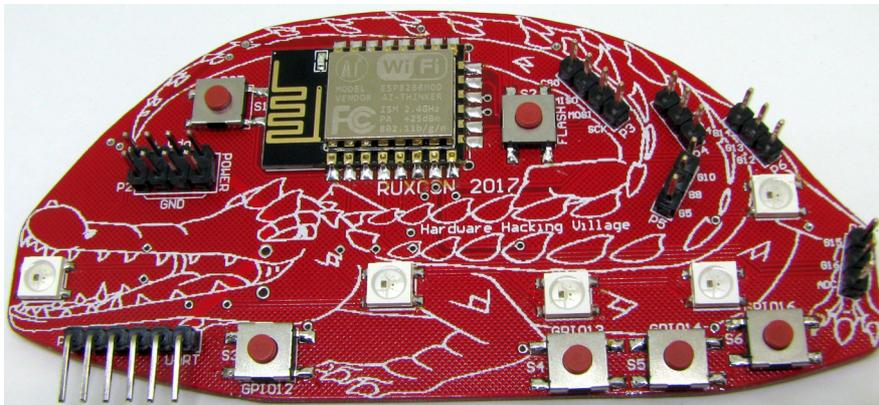
10. (OPTIONAL) The breakout headers are basically there to allow you to easily connect stuff to the ESP module on the badge, they are not essential for the function of the badge and can be omitted, it will also fit better in the pouch on your lanyard if you omit them :). P5 is the only one which can't readily be fitted “after the fact” (Due to the battery holder being in the way.) but if you needed to you could solder wires into the holes from the top of the board.
