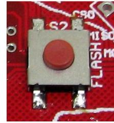
6. Next up is the two push button switches towards the top of the board. For these guys, tin one pad, tack the switch down, make sure it aligns with the other three pads (Note that the legs of the buttons “ride” the outside edge of the pads), then solder the rest of the connections and touch up the first if needs be.
